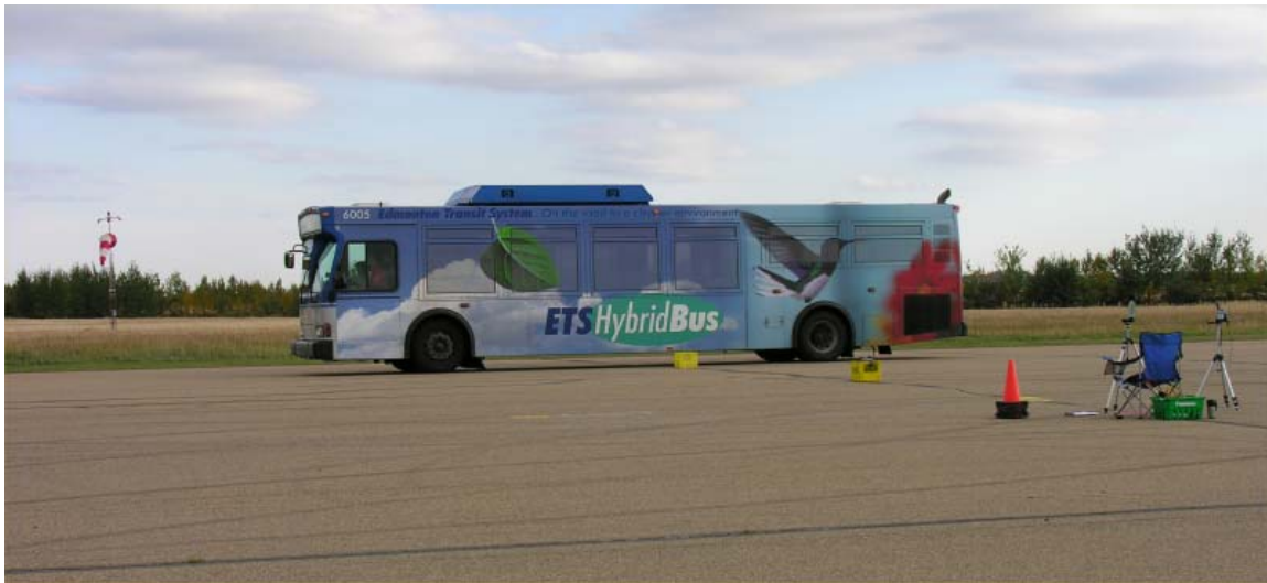
Figure 3. Hybrid Bus 6005 located at centre of test lane, 15 m from external observer station with sound level meter, anemometer and thermometer.
