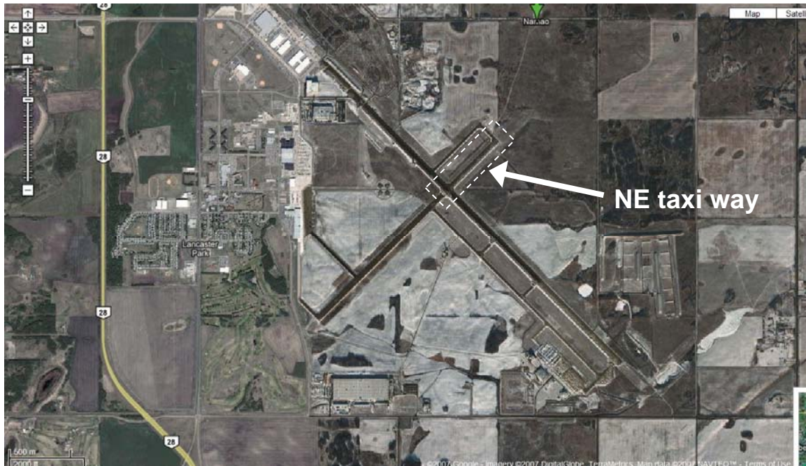
Figure 1. Satellite view of CFB Namao showing NE taxi way used for noise testing. Note that NE taxi way is approximately 600 m long and surrounded by flat agricultural fields.
